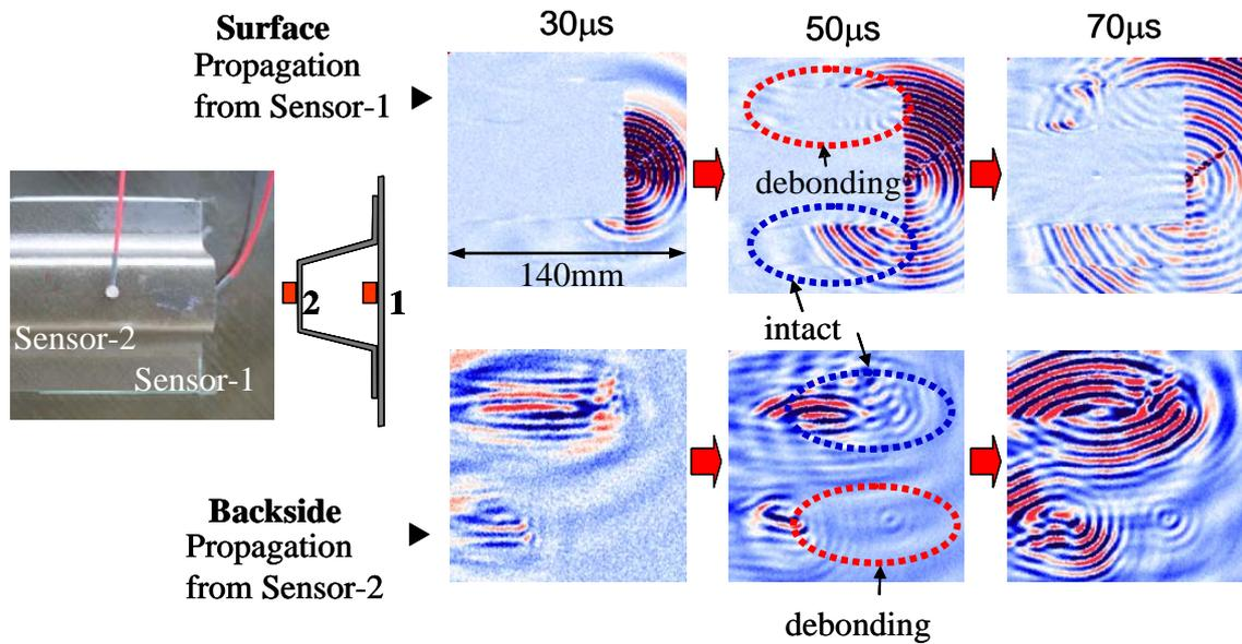
Fig.6 Visualization images of the ultrasonic propagation around a debonded area of the CFRP hat stringer sample
