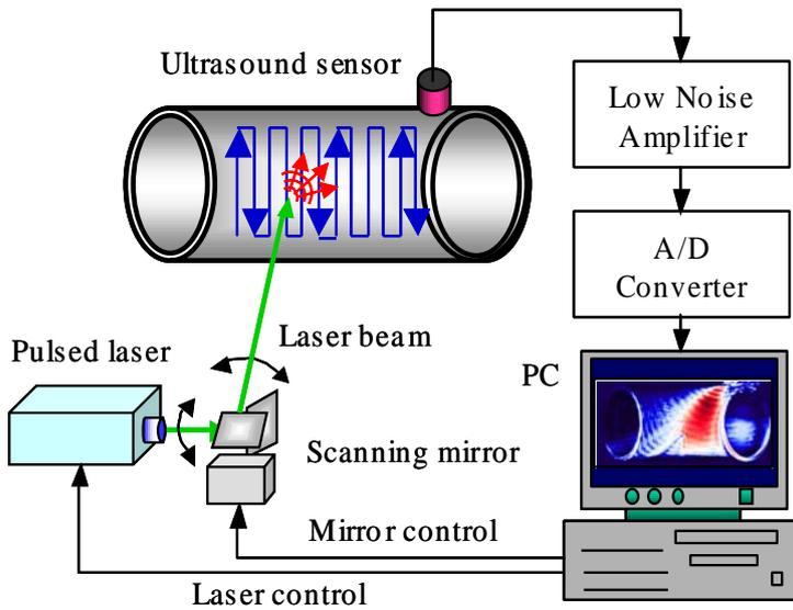
Fig. 1 LUV System Configuration
