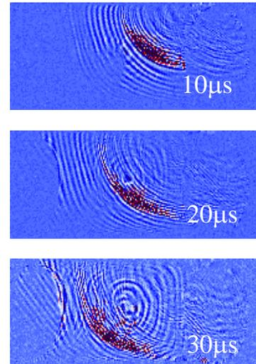
Fig.2 Ultrasonic propagation image of a stainless steel elbow with an inner corrosion
