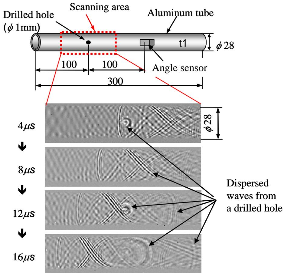
Fig.3 Ultrasonic propagation images of an aluminum tube with a small hole
