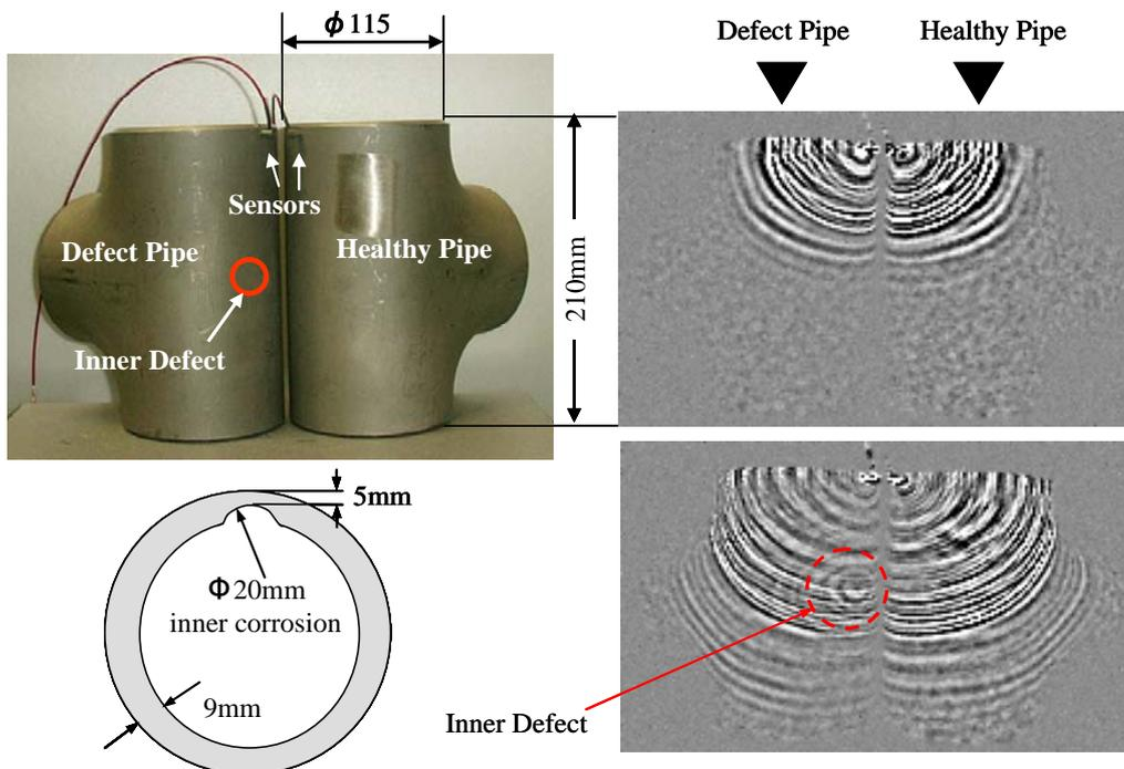
Fig.4 Ultrasonic dynamic Visualization images propagating on two T-shaped stainless steel pipes, the left one with an inner corrosion
