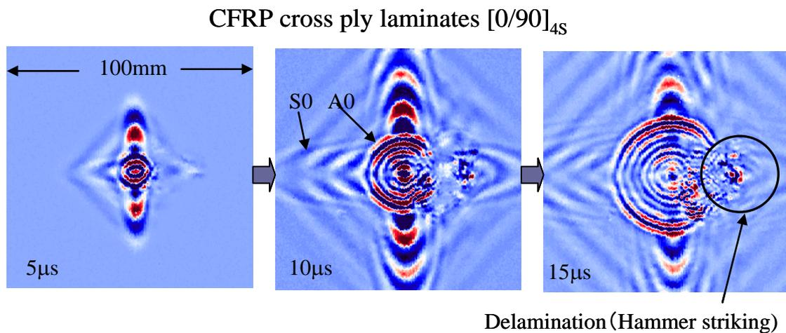
Fig. 5 Visualization of ultrasonic waves propagating on a CFRP[0/90]<sub>4S</sub> specimen having a delamination with a hammer striking.
