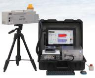
Small Laser Ultrasonic Visualizing Inspector (LUVI-LC1/LC2)
